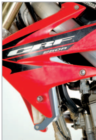
Knee damage: The CRD radiator brace works best against side impacts.
